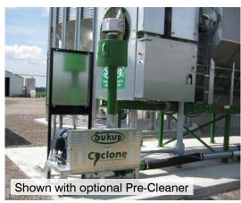
Positive displacement pumps and electric motors with shielded belt drive provide the air pressure for Sukup Cyclone Systems. Blower components are mounted on a heavy-duty, galvanized skid. An industrial air filter on the blower cleans the air entering the system. A filter restriction gauge lets you know when the filter needs to be cleaned.
