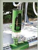
Compensator Valve maintains consistent line pressure to prevent grain damage.
