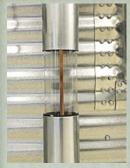
**Sight Glass** allows you to monitor grain flow and velocity.
