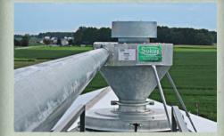
Galvanized 30" Dia. Cyclone is lined with long-lasting UHMW to protect the grain as it decelerates. All-galvanized construction and 11 ga. steel lining on the cone ensure long life. The Sukup cyclone is 66% larger than competing cyclones. The large diameter handles larger volumes of grain with less wear.
