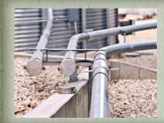
30°, 60°, and 90° elbows are designed with straight ends for better connections and less grain damage.
