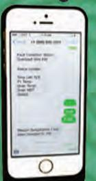
If the dryer shuts down, the GSM service sends a text message to a predetermined cell phone number, noting the fault. You can also text message the dryer to receive current dryer status, or adjust moisture, unload speed, and plenum temperature settings.
