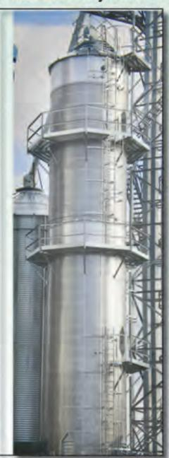
selects a desired drying temperature and the speed of the unload rotor is varied to obtain desired moisture output. Unload rotor speed is adjusted automatically based on the grain temperature in the bottom of the heat chamber or on the incoming and outgoing moisture content. If necessary, the unload rotor speed can be adjusted manually.
